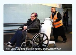
motorised devices that attach to manual H-frame wheelchairs of various sizes, and propel passengers safely on gradients with no force or effort required from the operator.
